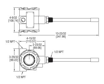
The **SERIES HHT** Hazardous Area Humidity/Temperature Transmitter takes accurate measurements in the harshest of environments. The explosion-proof model is offered with 4 to 20 mA output for humidity only. The intrinsically safe version is offered with 4 to 20 mA output for humidity and temperature, and do require an intrinsically safe barrier to meet hazardous area approvals.
