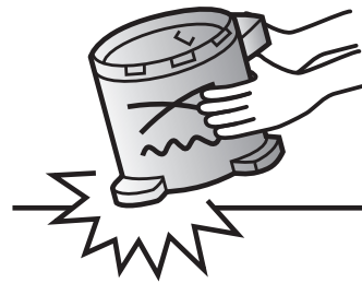
(2) Casually putting the unit down on a table or stand (put it down gently)
