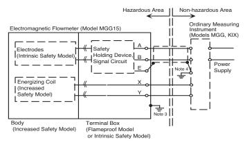
Note 1. Neither input power supply voltage to ground, nor voltage inside the ordinary measuring instruments should exceed 250V ac (50/60 Hz) or 250V dc during normal or abnormal operation.
