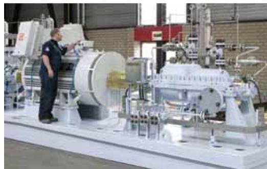
**ISO 21049/API 682 Seal Chambers** accommodate wet and dry gas seals, cartridge type single, dual unpressurized and dual pressurized mechanical seals.
