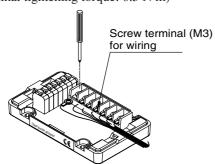
When the humidity output is the current output: Strip the sheath approximately 9 to 10 mm from the
