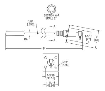
The SERIES AFG Flow Grid is a fundamental pressure-sensing device designed to sense velocity pressure in an air duct. When this output is connected to a suitable measuring instrument (i.e. manometer, pressure transducer, etc.) it may be used to determine air velocity or air flow rate.
