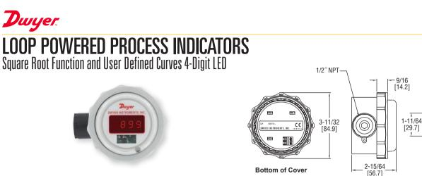
The **MODEL LPI** Micro-Pressure Based Loop Powered Indicator accepts a 4-20 mA input signal and displays the associated process variable such as pressure, level, flow, temperature, or relative humidity. The indicator is housed in a NEMA 4X (IP65) polycarbonate enclosure with a 1/2" female NPT side port. Users can quickly modify the instrument configuration via three push buttons on the front of the unit.
