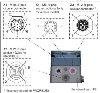
Fig. 22: PROFIBUS DP / DeviceNet; circular connectors and contacts - Type 8792
