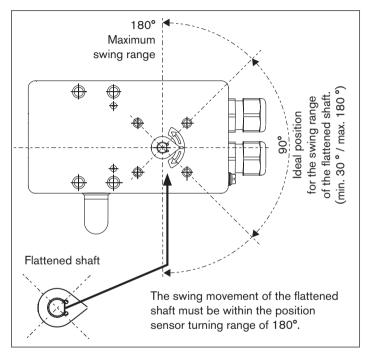
Fig. 11: Rotation range / anti-twist safeguard
