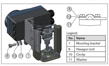
Fig. 9: Attach Type 8792/8793 with mounting bracket; for actuators with cast frame
