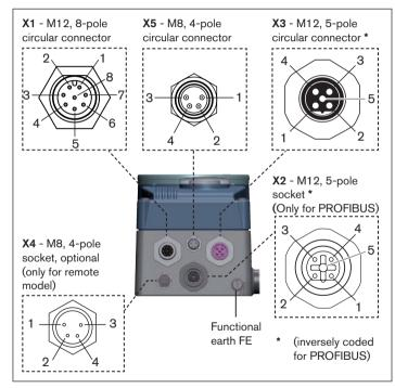
Fig. 23: PROFIBUS DP / DeviceNet; circular connectors and contacts - Type 8793
