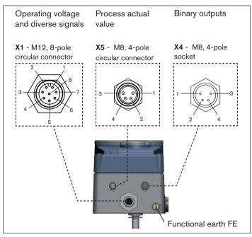
Fig. 19: Designation of the circular connectors and contacts
