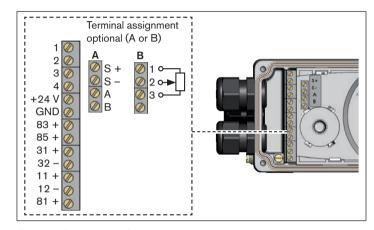
Fig. 21: Designation of the screw-type terminals
