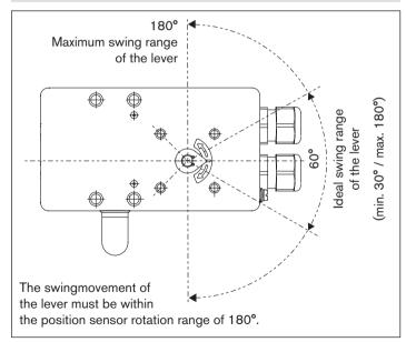
Fig. 7: Swing range of the lever
