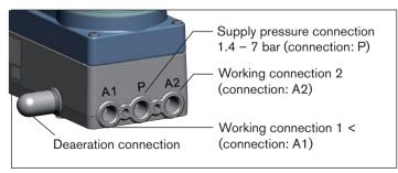
Fig. 15: Pneumatic installation / Location of the connections
