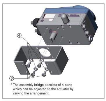
Fig. 12: Attach assembly bridge (schematic representation)
