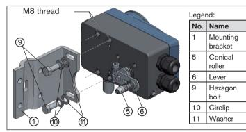
Fig. 8: Attaching mounting bracket
