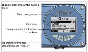
Fig. 4: Display elements of the setting level
