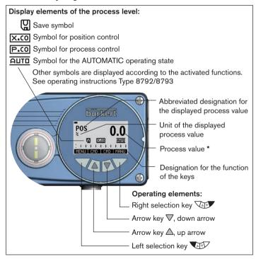
Fig. 3: Display elements of the process level; operating elements
