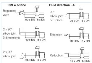
The flow rate sensor can be installed into either horizontal or vertical pipes.
