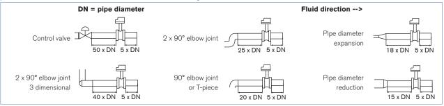
The flowmeter can be installed in either horizontal or vertical pipes, but following additional conditions should be respected
