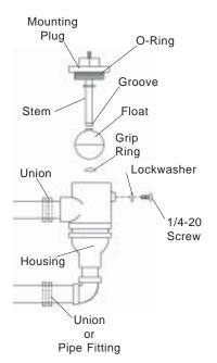
Standard single level units are supplied with SPST switch operation, N.O. (Dry).
