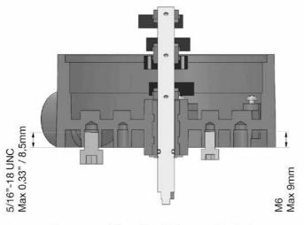
Max engaged thread length for mounting fasteners.
