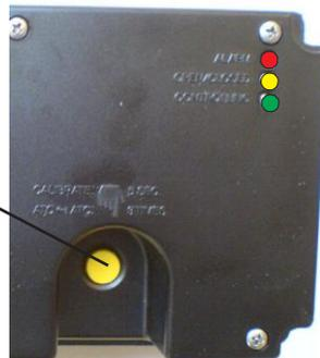
To indicate that a command is accepted, the three LED:s light up.
