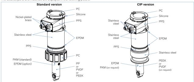
The detailed parts and materials are displayed in the following picture:
