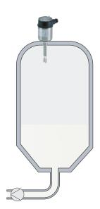
The processes in food processing tanks such as e.g. for milk have a high demand to the installed technology. High pressures and temperatures are caused during sterilization and cleaning of the tanks. The installed level sensors must meet the requirements of the hygienic construction. The harmlessness of all wetted materials must be proven and optimum cleanability must be ensured by hygiene-technical design.
