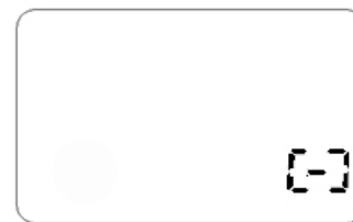
Meter Installed Backwards
