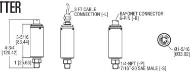
The SERIES 644 High Accuracy Pressure Transmitter is a robust transmitter designed for high accuracy pressure applications. Boasting an accuracy of  $\pm 0.05\%$  FS RSS (<±0.25% TEB), the 644 is intended for precise measurements in the critical applications.
