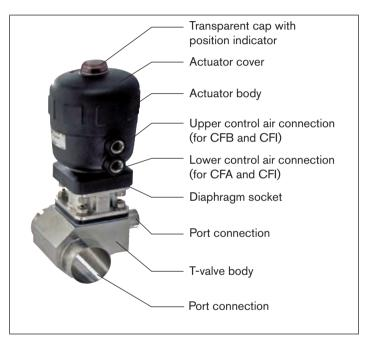
Fig. 22: Structure and description Type 2032
