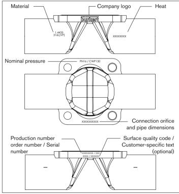
Fig. 3: Labeling of the tube valve body (VP)
