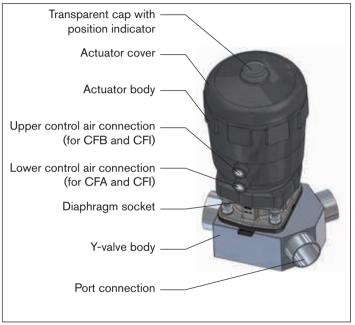
Fig. 24: Structure and description Type 2037
