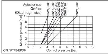
Fig. 11: Control function I, PTFE elastomer diaphragm, actuators ø 40 - 80 mm
