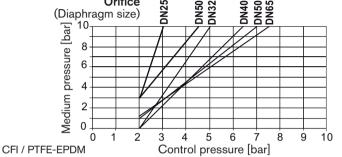
Control function I, PTFE EPDM diaphragm, Fig. 20: actuators ø 80 – 125 mm
