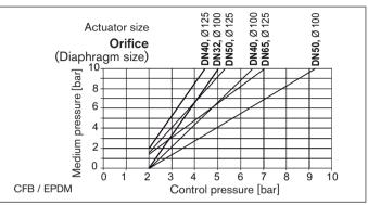
Control function B, elastomer diaphragm, Fig. 6: actuators ø 100 – 125 mm
