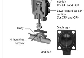
Fig. 32: Replacement of diaphragm
