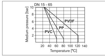
Fig. 4: Graph of medium pressure / Medium temperature
