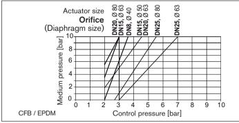
Control function B, elastomer diaphragm, actuators Fig. 5: ø 40 – 80 mm
