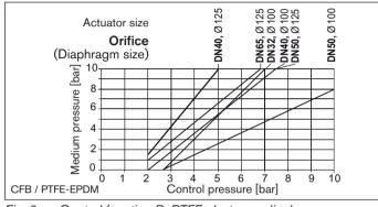
Fig. 8: Control function B, PTFE elastomer diaphragm, actuators ø 100 – 125 m
