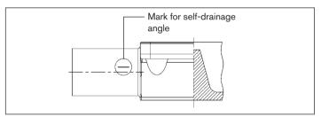
Fig. 26: Mark for the correct installation position
