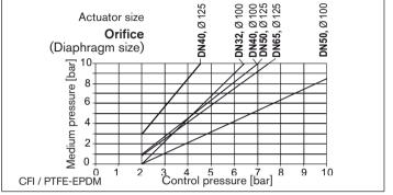
Control function I, PTFE EPDM diaphragm, Fia. 12: actuators ø 100 - 125 mm
