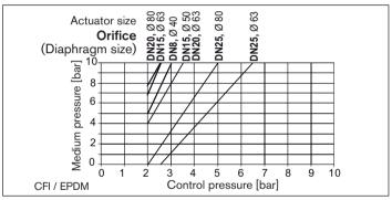
Fig. 9: Control function I, elastomer diaphragm, actuators ø 40 – 80 mm
