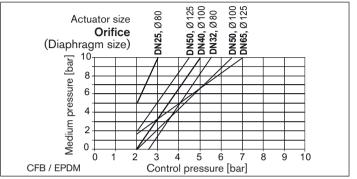
Fig. 14: Control function B, EPDM diaphragm, actuators ø 80 – 125 mm
