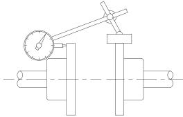
CHECKING ANGULAR MISALIGNMENT Figure 4 – Angular Misalignment
