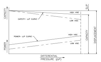
Figure 6 – D.P. vs. capacity relationship
