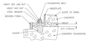
Figure 1 – Grout Installation
