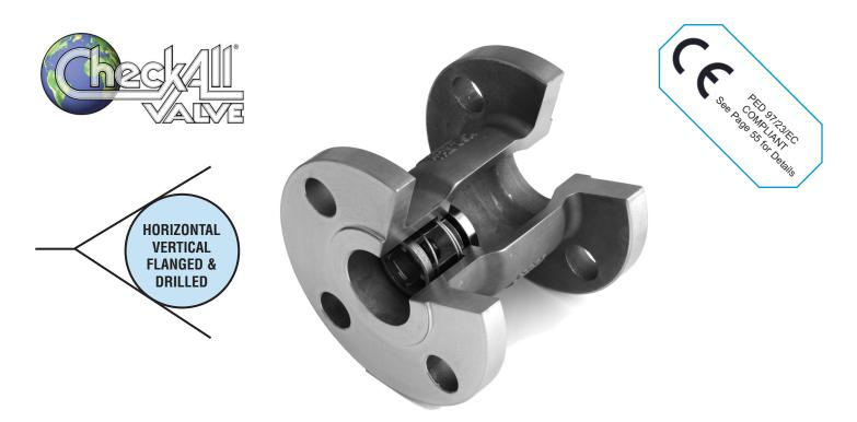
The **Check-All® Flanged & Drilled (HV)** check valve is a one piece cast body valve with ASME/ANSI B16.5 Class 150 flanged ends. The HV series valve is used when higher flow rates and lower pressure drops are required. The valve is available in sizes 1 inch through 10 inches and standard materials of CF8M (cast 316 stainless) and WCB/WCC (cast carbon steel). The HV series valve is designed for use with mating ANSI Class 150 flanges. Other materials are available upon request.
