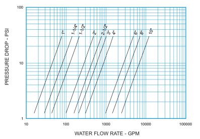
**Note:** All flow curves and Cv values presume the valves are fully open with 1/2 PSI cracking pressure springs. Consult the factory for more information.
