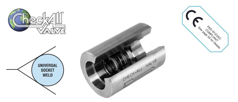
The **Universal Socket Weld (US)** check valve is a one piece body machined from bar stock with socket weld ends and is designed for a minimum pressure drop. It carries rugged, dependable Check-All<sup>®</sup> trim and there are a wide variety of seat materials and cracking pressures to choose from. The socket ends are machined to ASME/ANSI B16.11 dimensions. The US valve can also be used as a low pressure relief valve or vacuum breaker by using the desired spring settings.
