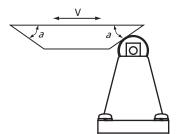
When using with the dog speed (V) faster than 0.3 m/s, change the dog angle ( $\alpha$ ) according to the table below.
