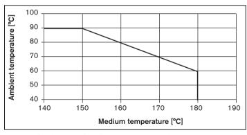
Fig. 1: Combination of medium temperature / ambient temperature
