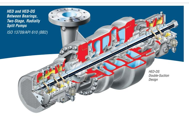
Fully compliant with the latest edition of ISO 13709/ API 610 (BB2), the Flowserve HED pump is a between bearings, radially split, two-stage, single-suction hydrocarbon processing pump. The similarly configured HED-DS boasts a double-suction, first-stage impeller for services with very low NPSHA or higher flow rates. Both pumps are CE compliant and engineered to provide safe, reliable operation in the elevated temperatures experienced in refining and power applications.
