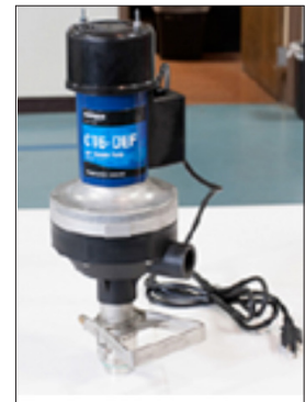
115V CT6 DEF Pump with Micro Matic valve
