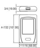
The **MODEL DW-DATAPAD** Handheld Portable Data Viewer configures and reads data from up to 500 DW-USB data loggers and utilizes a 2.8" full color TFT touch screen display. Data can be displayed as a trend graph or a statistical summary, and can also be transferred to a computer using the provided cable and Windows<sup>®</sup> based software. Model DW-DATAPAD features a rechargeable lithium battery and has an average life of 5 to 8 hours under constant use.
