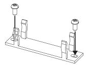
(2) Mount the main unit on the mounting bracket.
