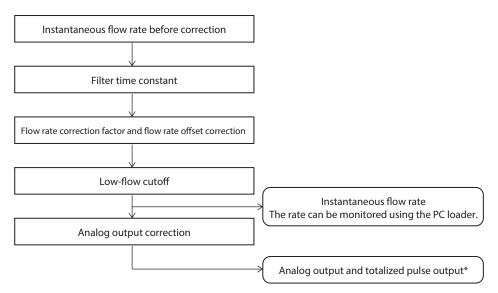
\* By setting "DO function" to "3" (Totalizer pulse output) using the PC loader, totalized pulse can be output.
