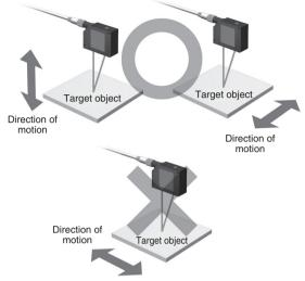
Install the sensor in the same manner even if the color or surface condition of the target objects changes greatly.
