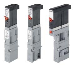
The solenoid valve Types 6524 and 6525 consist of a 6144 flipper pilot valve and a pneumatic seat valve. The principle allows switching of high pressures together with low power consumption and fast response times. The pilot valves are equipped with manual override as a standard.
