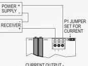
CURRENT OUTPUT -WIRING AND P1 SETTING
