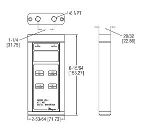
The SERIES 490A Digital Manometers are versatile, hand-held, battery operated manometers available in several basic ranges for positive or positive differential pressure measurement and can tolerate most liquid media compatible with 316LSS. A new feature added to the Series 490A is a field adjustable damping, which allows the user to choose the level of display averaging rate corresponding to the fluctuation level common in many applications.
