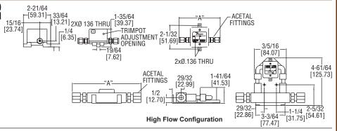
The SERIES TFP-GV Gas Flowmeters utilize a turbine wheel and electro-optical detection to convert flow rates into a linear 0 to 5 VDC output signal for recording and data logging. Couple this unit with a Series FIV Flow Totalizer for a remote flow monitoring display. A power adapter or mating cable assembly is required for operation.
