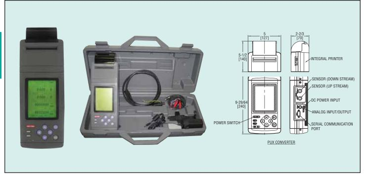
Series PUX Portable Ultrasonic Flowmeter Converters are paired with Series PSX2 sensors in order to utilize the transit-time difference for measuring flow rates in pipes from the outside. It is a compact and lightweight instrument incorporating the latest electronics and digital signal processing technologies, realizing high performance and easy operation. This portable unit is designed for 5 hours of continuous operation with its built-in battery, which only requires 3 hours to recharge.
