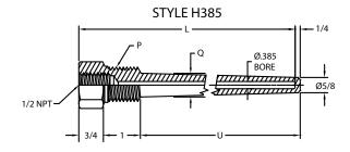
(\*) Thermowells with an overall length of 42" or less are machined from SOLID BAR STOCK. Thermowells with an overall length greater than 42" are constructed using a welded design and are available in straight, stepped or tapered design. However, for tapered only the last 16" are tapered.
