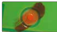
Reject mark *The reject mark is applied to the gold pattern using an oil-based red felt pen.
