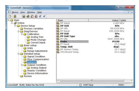
The temperature sensor can be selected from the following two types.
