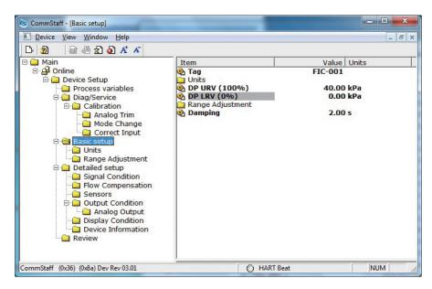
Note: When using SFC or CommPad, if the LRV is changed, the URV will change by the same amount so that the span does not change. However, when using CommStaff, the URV does not change if the LRV is changed.
