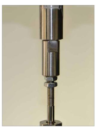
Fig 6.7 Connection of valve shaft and actuator shaft
