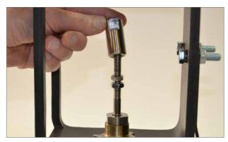
Fig 6.4 Coupling attachment to valve shaft
