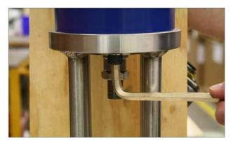
Fig 6.6 Secure mounting fixing
