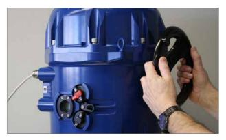
Fig 6.3 Manual operation of the actuator
