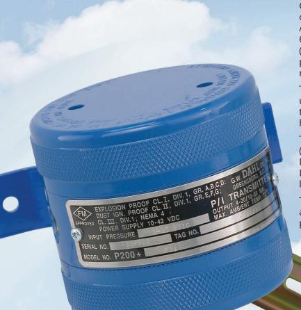
ControlAir's P200 and P290 P/I transducers represent outstanding value in pneumatic to current technology. All solid state circuitry converts standard 3-15, 3-27 or 6-30 psig instrument air into 4-20 or 10-50 mA outputs (4-20 mA only for FM and CSA approval) with uncompromising accuracy and durability. Custom pressure ranges are also available.
