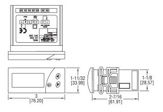
The Series LCT316 Low Cost Digital Timer provides accurate countdown timing for a variety of applications. The timer can be triggered remotely using the digital input terminals or locally via the set button. Time intervals can be set up to 999 minutes or seconds. The Series LCT316 has an internal buzzer to alert when the time interval has expired.
