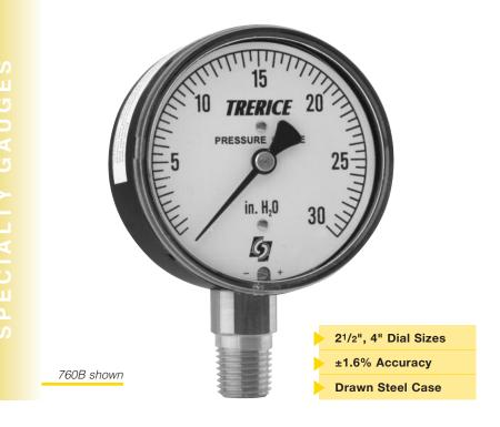
The Trerice **760B** Low Pressure Gauge is designed to accurately measure extreme low pressure conditions. This pressure gauge employs a diaphragm capsule sensing element to measure the low pressure. Case material is drawn steel with brass wetted parts.
