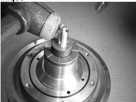
Figure 6-28: Guardian H series bushing alignment technique
