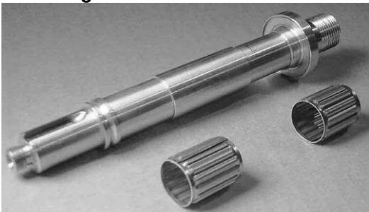
Figure 6-19: Group 1 shaft with unmounted tolerance rings
