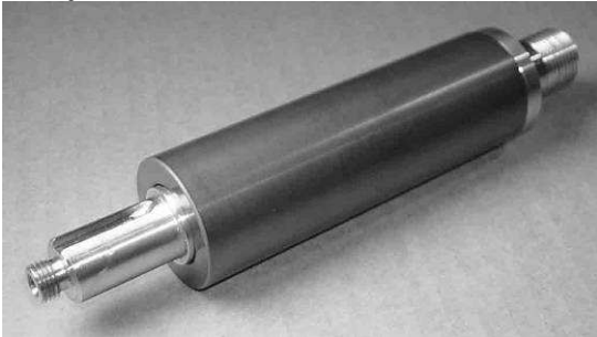
Figure 6-17: Group 1 shaft with mounted tolerance rings
