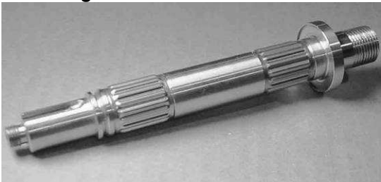
Figure 6-17: Group 1 shaft with mounted tolerance rings
