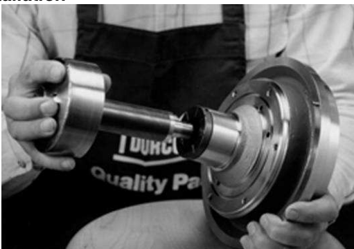
Figure 6-36 Inner magnet/shaft assembly installation
