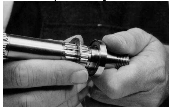
Figure 6-29: Pump shaft with gasket
