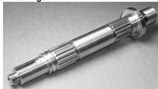
Figure 6-30: Group 1 pump shaft with mounted tolerance rings
