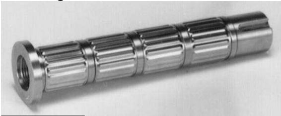
Figure 6-31: Group 2 pump shaft with mounted tolerance rings
