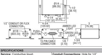
The SERIES WD Water Detectors and Sensor Tapes is designed for dependable detection of water presence even of low conductive liquids. The water sensing tape attaches to module and if any liquid comes in contact with the tape the resistance is changed and the alarm will be triggered. The sensing tape is 1" wide and can be bought in lengths of 5, 10, 15 and 25' and is powered by 24 VAC or 24 to 30 VDC.
