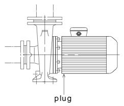
Fig. 1 Evacuation of condensation water
