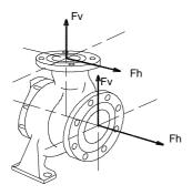
Forces and moments values are applied to the whole flanges and not flange-by-flange. For their sharing out on the pump flanges, refer to standard NFCR 13 931.
