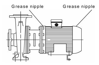
Fig. 2 Bearing lubrication
