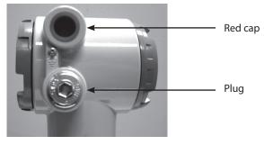
(2) Remove the red cap from the wiring port. When leading out the wiring from two ports, remove the plug also.
