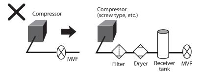
As shown in the above figure, provide the devices eliminating the foreign matters such as oil, water and iron powder, and install a receiver tank as the measures against pulsating flow ; at the upstream of MVF series.
