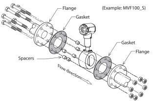
To mount this device, sandwich it between two pipe flanges (wafer mounting). Note that spacers should be used to prevent displacement during mounting. The use of spacers enables proper alignment of the piping and this device. Be sure to use the spacers.
