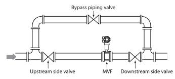
• Provide a straight pipe section in upstream side and downstream side of the installation location.
