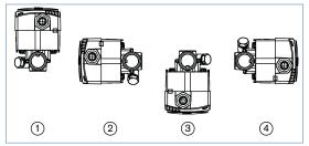
If the absence of any air bubbles cannot be guaranteed, the device should be fitted on a horizontal pipe, with the electronic enclosure facing down. This way, the bubbles will not interfere with the circulation of ultrasound waves.
