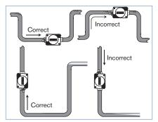
Minimum upstream and downstream distances are not necessary.
