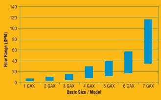
\* For a quick selection of the GAX pump model corresponding to the desired flow rate, refer to the chart above. The ranges shown are based on typical viscosities and speeds and assume a zero differential pressure. The chart's purpose is to direct the user to the appropriate performance curve, not to be a substitute for it.
