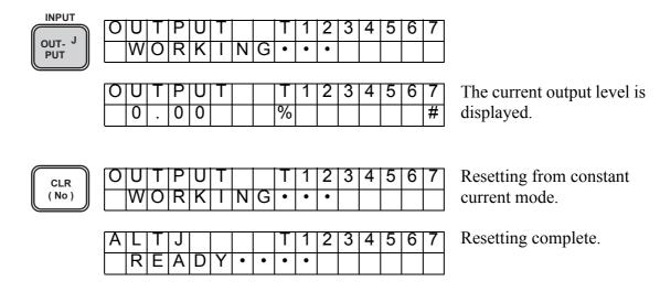
**~Note** The "#" will disappear, indicating that the transmitter has been reset from the constant-current mode.
