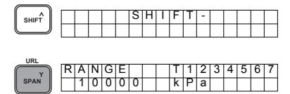
• Check that the upper limit value specified as the configuration data is within the adjustable range of the transmitter. If the value is not within range, replace the transmitter with another transmitter which can handle a wider range.
