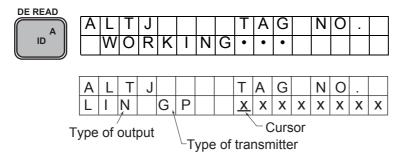
When the transmitter is shipped from its manufacturer, the tag no. is set to "xxxxxxxxx"
