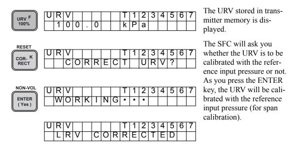
After the above calibration of the LRV and URV are finished, save the data into the nonvolatile memory (NVM). Refer to Note on page 3-4.
