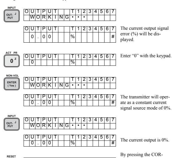
If the meter reading is lower than 4mA or IV (with a voltage drop resistor of 250 ohms), proceed as follows:
