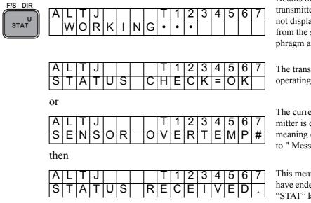
Details of failure status of the transmitter sensor section are not displayed. Deduce them from the statuses of the diaphragm and sensor.
