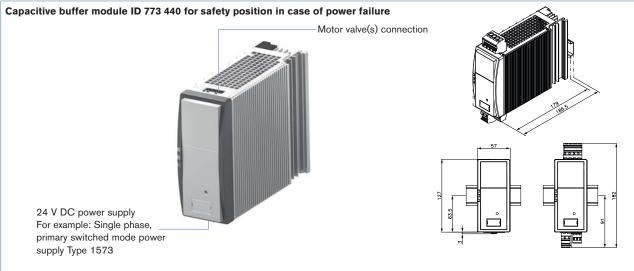
In the case of power failure the valve can be moved into a safety position, using the capacitive buffer module. In case of power failure the buffer module maintains the power supply for a few seconds at 18 V DC. The reduced input voltage is detected by the valve, and the safety position is established. Up to three type 3280 valves and two type 3285 valves can be connected to one buffer module.
