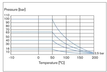
Fig. 2: Pressure-temperature graph stainless-steel valve body (Types 2651, 2654, 2654 Hygienic, TKU 001)
