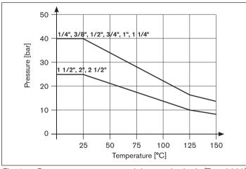
Fig. 1: Pressure-temperature graph brass valve body (Type 2660)
