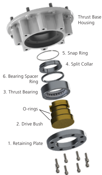
Fig. 5.1.4 F25 & F30 base assembly
